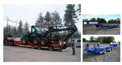
Designed specifically to carry forestry forwarders and forwarders by commercial towing vehicles, Chieftain's jumbo forestry trailer is both a reliable and practical transport solution
