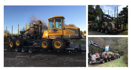
With its heavy duty wheel arches, low bed height and front and rear loading ramps, the Chieftain forestry trailer is specifically designed for the safe and efficient transportation of large forestry harvester and forwarder machines
