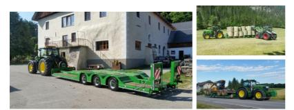
With a loading height of 350mm, the Chieftain Low Ride Forestry trailer is specifically designed to safely transport large forestry harvester and forwarder machines in regions where height restrictions mean that overall loaded height must be kept to a minimum
