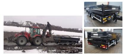
Chieftains 3 way tipping Road Rail Trailer can be used for distributing ballast/material in 3 different directions ie both sides and to the rear
