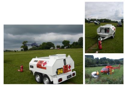
Middle of the range at 300 gallons / 1450 litre litres, Chieftain's UN approved bunded towable Aviation Fuel Bowser complies with all UN fuel transportation regulations and has full EU type approval. This permits the safe and legal transportation of aviation fuel on the open highway. The tough chassis and high speed twin axles ensure ease of towing for the driver, and with a lockable cabinet and ball hitch lock ensure a secure method of bringing fuel to and from site
