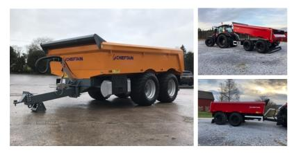
The Chieftain SB14 Dump Trailer is designed for the transportation of materials behind agricultural tractors for up to 40km/h. By choosing the option of an invisible rear door the trailer becomes multi purpose for the loading and transportation of small machinery
