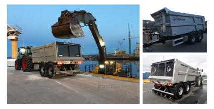
The Chieftain SB25 Fast Tow Dump Trailer is designed for the transportation of materials behind high speed tractors and Fastracs for up to 60km/h. By choosing the option of an invisible rear door the trailer becomes multi purpose for the loading and transportation of small machinery
