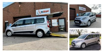
2016 Ford Grand Connect Flexi has been converted by McElmeel Mobility Services with a lowered floor to make it fully wheelchair accessible.
