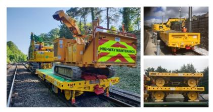
The Chieftain 3m and 4m Rail Trailers are the shortest in our rail trailer range. These trailers are ideal for mainline rail work and can be manufactured to suit narrow gauge, standard gauge or broad gauge, track gauges. Trailers are approved for RIS 1530 Issue 6 (UK), DB netz (Germany) & I-PLM-5001 (Ireland)
